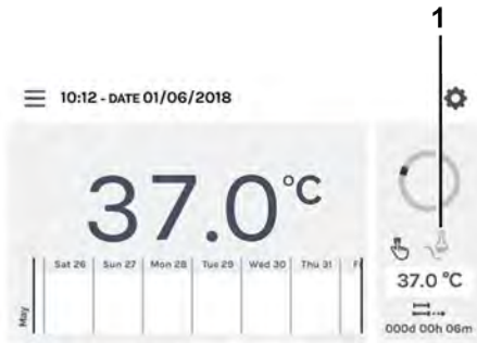
Fig. 64: Main screen, temperature drop exists, but is inactive
